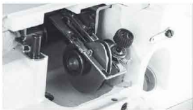
Hidden outer thread cam
