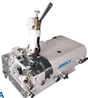
SK801 削皮机 Leather skiving machine Leather skiving machine with circular knife is suitable for edge skiving and whole surface skiving of any kinds of leather, such as plastic cloth, synthetic leather, felted wool and rubber for shoes, caps, bags, garments, belts, gloves and sports goods etc.
