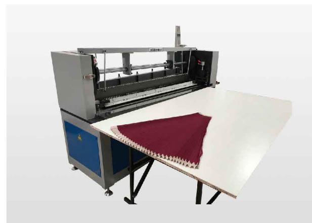
JK-F516D 电脑打折机 Computerized fabric pleating machine (for skirt)
